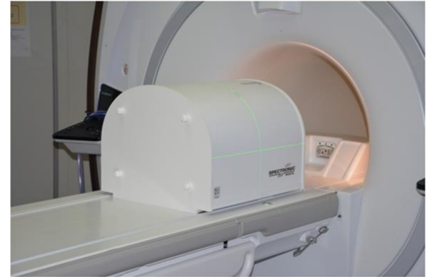
Figure 1. The commercially available phantom from Spectronic Medical AB is designed to assess geometric accuracy. It was placed on the MRI table without table top. Lines on the phantom surface were used to align the phantom using the built in laser positioning system on the MRI.
